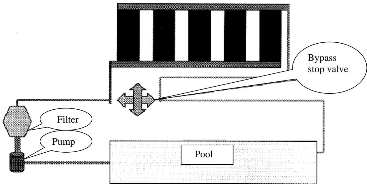
Find a suitable location for connecting the solar system to the water circuit between the filter and pool. See Fig. "F".
