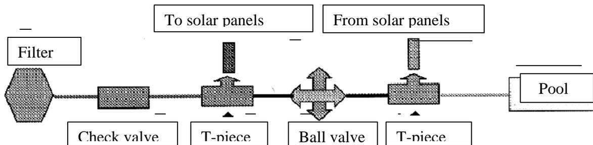
The last thing one has to do is to connect the pipes from the solar panels to the filtration system. These pipes should have at least 55mm and/or 63 mm in diameter. Where possible, our recommendation is to bury the whole system's lines in earth or lead them through interiors. Where the pipes are not buried, make sure they are fastened properly, embedded (best option) into the wall. It is vital as the pipes, when full of water, are very heavy and might suffer damage.
