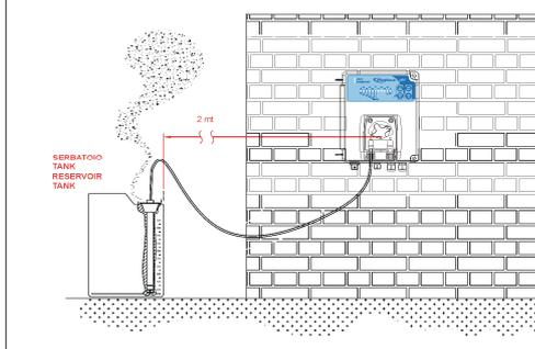
*Make sure that the injection pressure is below 1.5 bar.*
