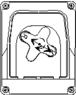
Position the roller at 10 and 20, turning it in the direction of the circular arrow.
