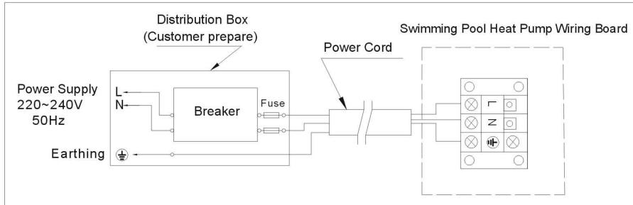
Note: The swimming pool heater must be earthed well.
