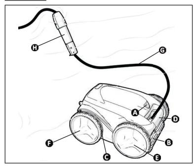
(A): Filter access hatch lock
