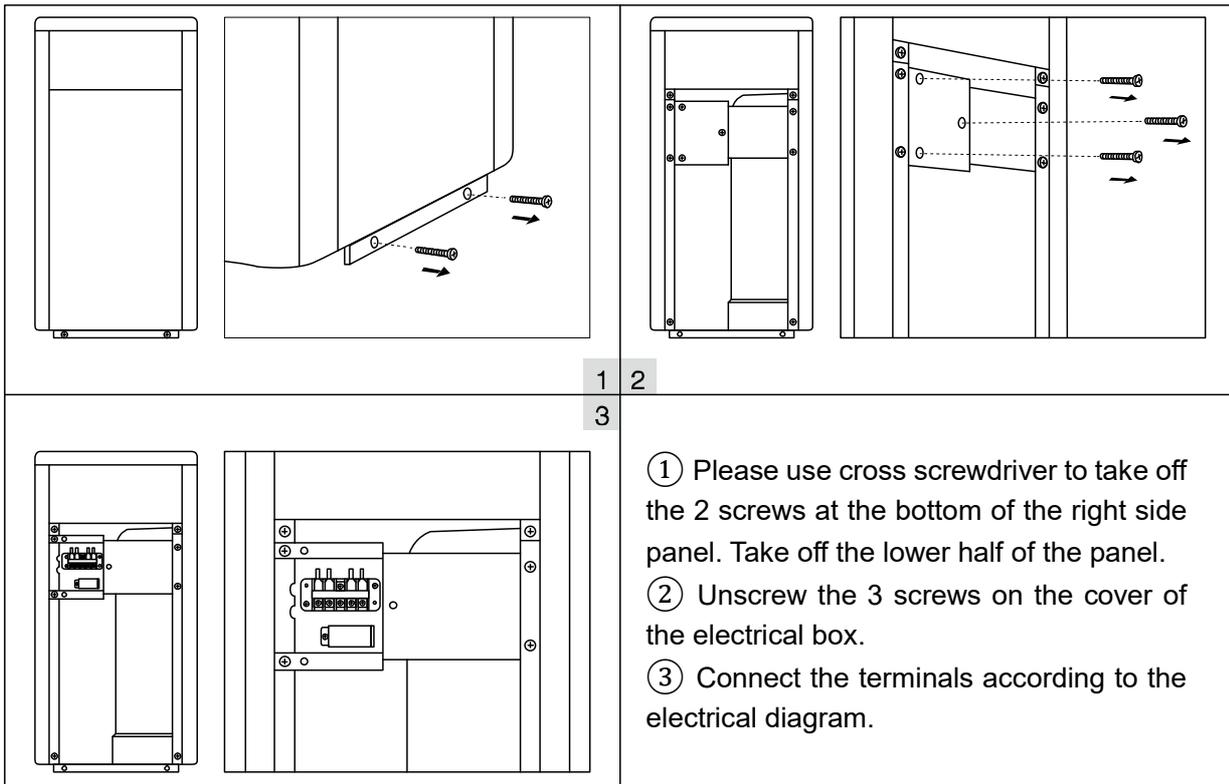
*Note: For IPHCR15-33 model, please open the back panel for power connection. The operation is the same as above.*
